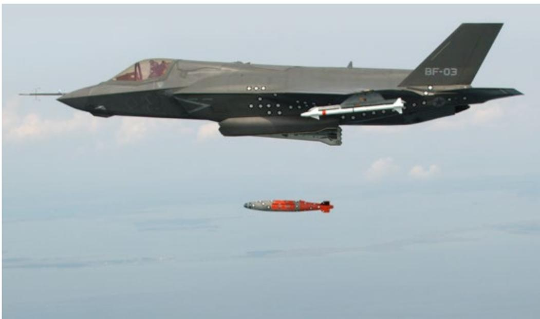
© 2012 U.S. Navy photo courtesy Lockheed Martin/Andy Wolfe/DoD: 120808-O-GR159-003, Naval Air Station Patuxent River, Md. August 8, 2012) F-35B test aircraft BF-3 completing the first aerial weapons release for any variant of the aircraft.
